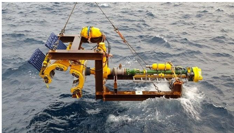
Figuur 5-15: Hot tap tool ( https://www.statsgroup.com/resources/video/suretap-subsea-hot-tapping-pipeline-rerouting )
