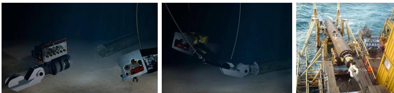
Figuur 5-11: Pipeline Retrieval Tool (P.R.T) Statsgroup ( https://www.youtube.com/watch?v=wFT-mmi9nkw )
