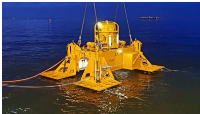
Figuur 5-12: Onder water lassen (hyperbaric welding) DCN ( https://dcndiving.com/international-accolades-for-dcn/ )
