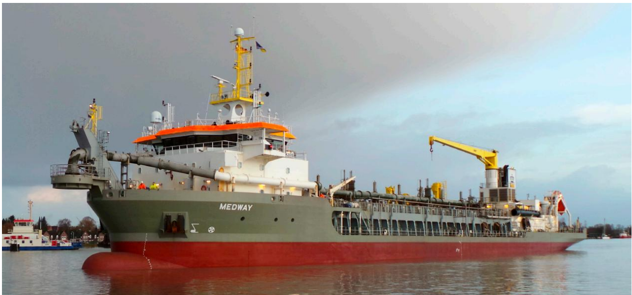
Figuur 5-5: Medway - Trailing Suction Hopper Dredger. Capaciteit: 7,516 m 3 . ( https://boskalis.com/media/etzomdxk/medway.pdf )
