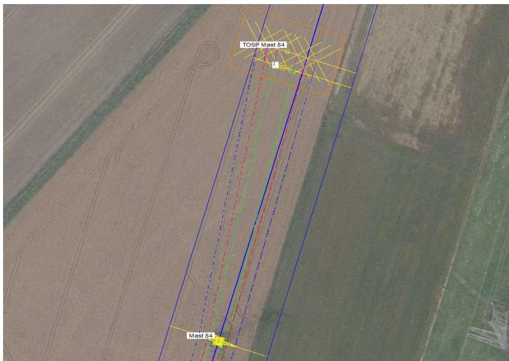
Figure 3-14 RSD-MDK150 Mast 84 (D+0) span to temporary OSP in PLS-CADD view
