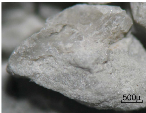
pict. B480-176-20: RNMU: A4f non argillaceous, non calcareous sacharoidal dolomite with gypsum nodule
