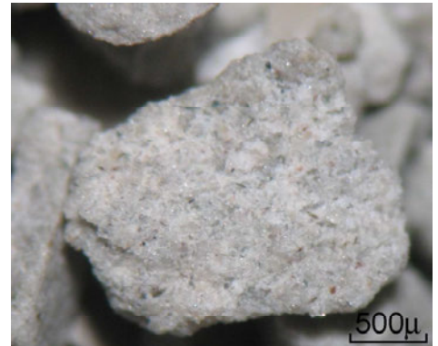
pict. B483-143-20: RNMU-A2c siltstone with calcareous / dolomitic cement and very fine mica
