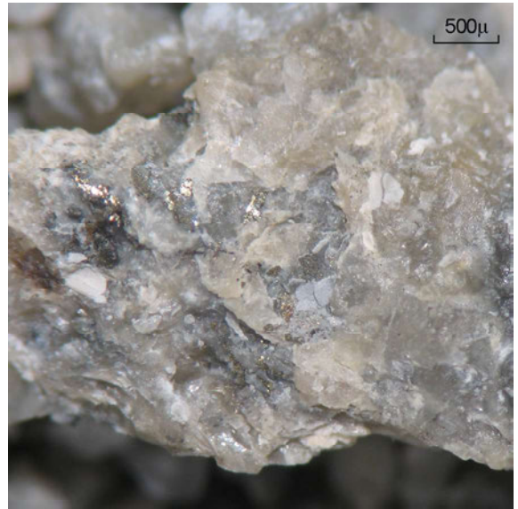
pict. B478-121-20: SK-D bioclastic limestone with pyrite
