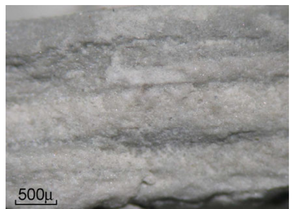
below pict. B480-159-20: RNMU-B1 sacharoidal argillaceous dolomite with thin argillaceous laminae
