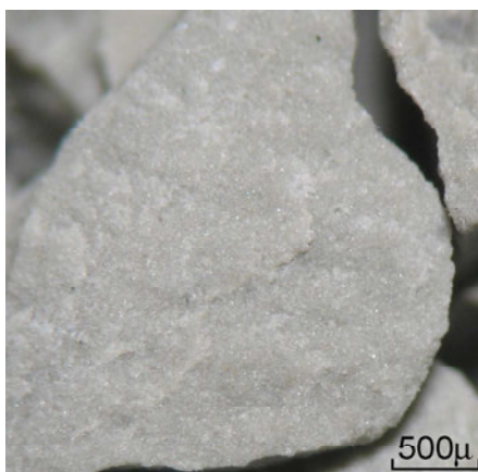
below pict. B154a-210-20: RNMU-B1 calcareous cryptocrystalline dolomite
