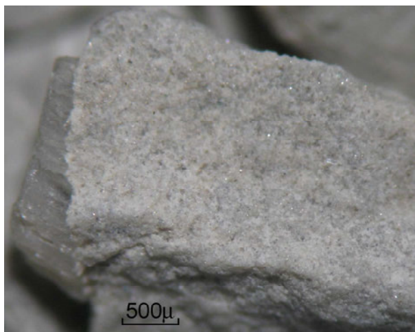
pict. B480-117-20f: RNMU-B4 sacharoidal dolomite with attached gypsum vein
