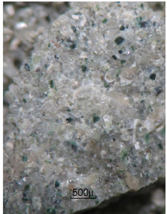
pict. HEN-01-50-20 very fine to medium grained sandstone with mainly quartz cement, resembling Brussels Sand Mb.lithology
