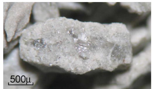
pict. B483-139-20: RNMU-A3 silty dolomite with mica and gypsum crystals/nodules
