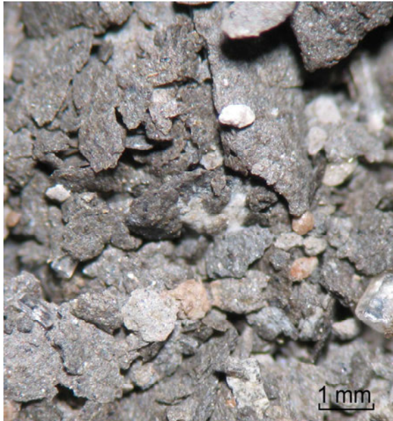
pict. B480-112-10: ATRT-A brownish grey claystone, with very fine organic matter/ plant fragments and gypsum crystals
