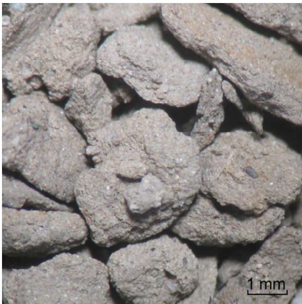
pict. B175-120-10: N1b light to medium brown to slightly reddish brown very silty to very fine sandy clay, grading argillaceous sand
