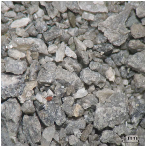
pict. B478-110-10: SK-D overview of sample of bioclastic limestone
