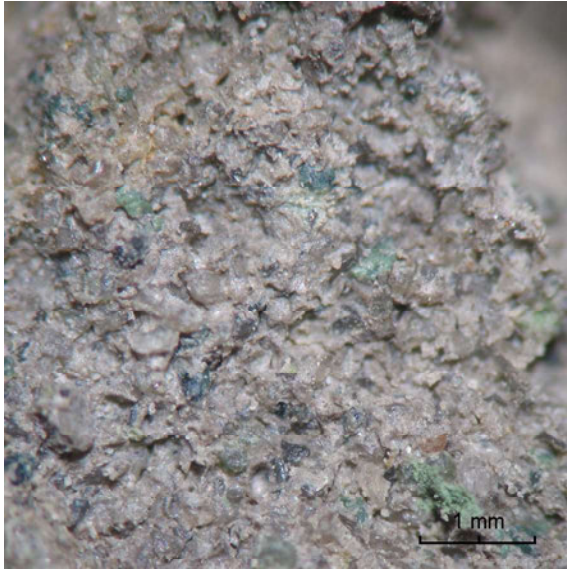
pict. B480-74-40c: N-1a light brown very fine to medium sand, with argillaceous matrix, glauconite and dark organic particles
