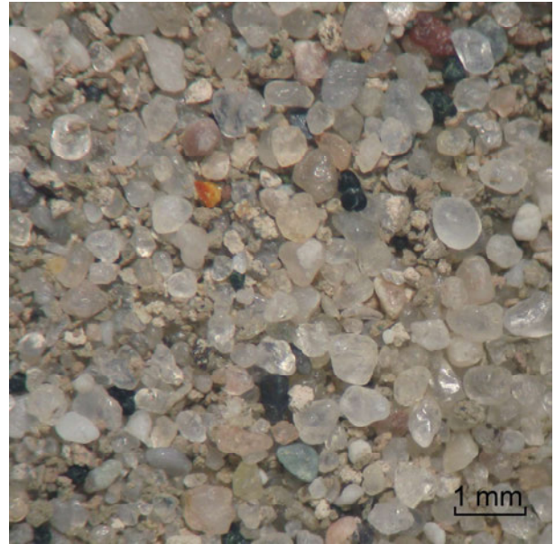
pict. B175-60-10 (washed sample) fine to coarse quartz grains with glauconite
