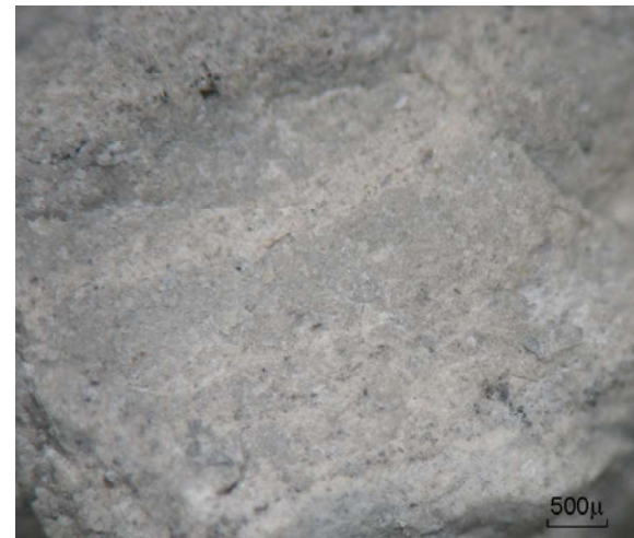
pict. B478-170-20: SK-A micritic argillaceous limestone with plant fragments
