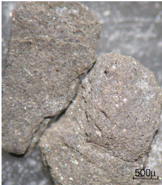
pict. B480-112-10: ATRT-A brownish grey claystone, with very fine organic matter/ plant fragments and gypsum crystals
