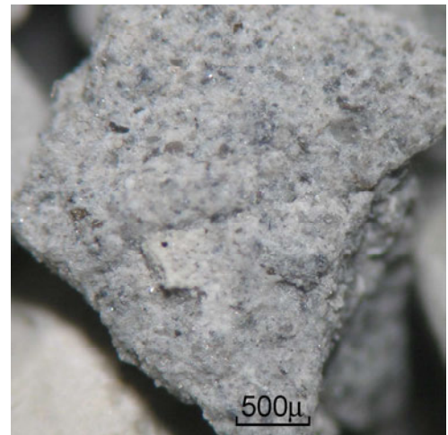
pict. B483-130-20: RNMU-A4b silty calcareous dolomite with mica
