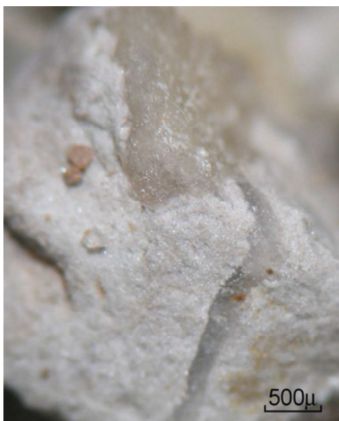
pict. B483-161-20: RNMU-A2a slightly saccharoidal dolomite with gypsum nodules and veins
