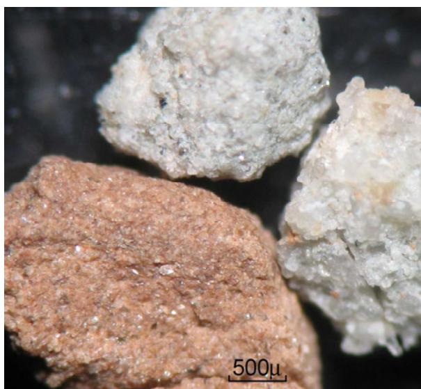
pict. B483-294-20: RNROU-C1 siltstone / very fine sandstone with dolomite / gypsum / anhydrite cement
